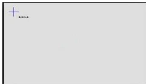
Use a pen included with the whiteboard and touch the centre of each crosshair (and hold it for a few seconds). As soon as the four registration points have been identified, the calibration process will be completed.
